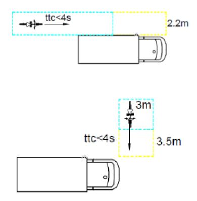
When the Blind Spot Information System identifies that a collision is imminent, for example if the vehicle turns toward the VRU,
