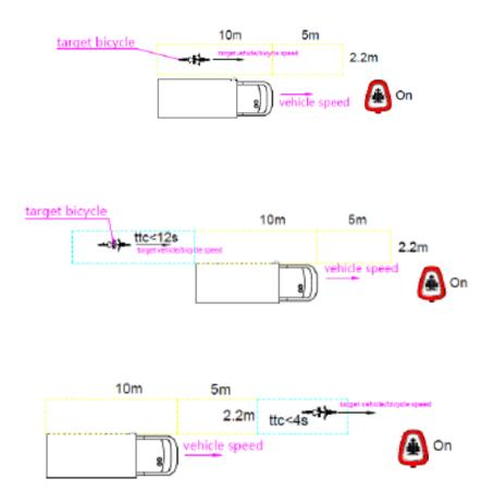
It shall also **inform** the driver about approaching VRUs while the vehicle is stationary before the VRU reaches the vehicle front, considering a driver reaction time of 1.4 seconds.
