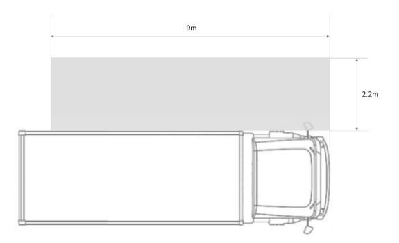
The system shall also be capable of providing collision warnings whenever it is active and a VRU is detected, and the system calculates that a collision is imminent based on the trajectories of the vehicle and/or the VRU.
