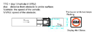
The collision warning signal shall be easily understandable for the driver to relate the signal to a potential collision.
