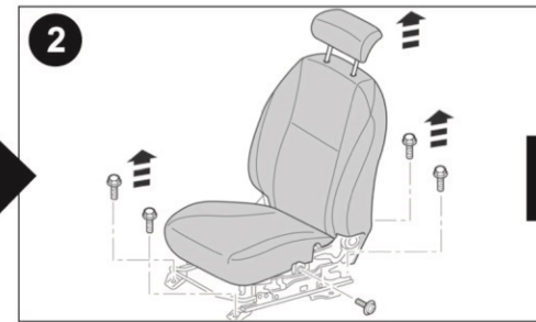
Remove seat and place on work bench for easy access.
